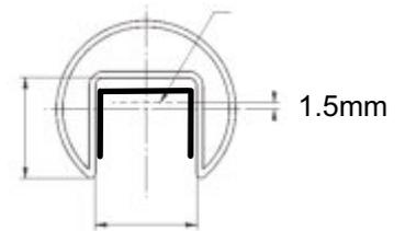
3. Nutrohr vierkant, 40x40mm oder 60x40mm dicke 1.5mm, Nut BxT mm 24x24mm
